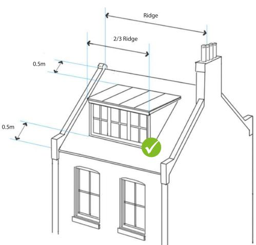
Dormer roof extensions should be subordinate to the original roof.
