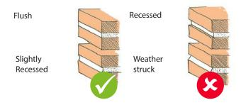
A flush or slightly recessed mortar joint is the most appropriate.
